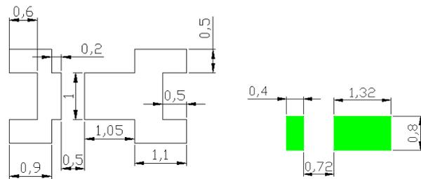
◇ Recommended solder pad design for heat dissipation (EMC T34 Series -3020)
