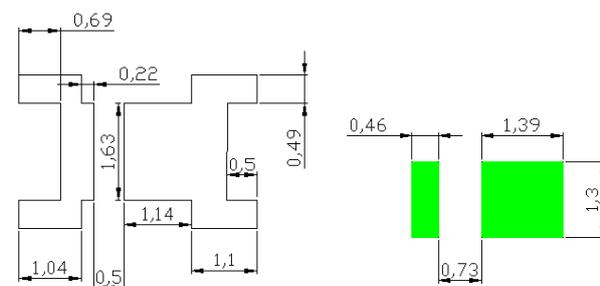
◇ Recommended solder pad design for heat dissipation (EMC T3C Series -3030)
