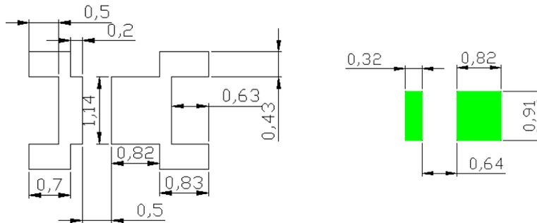
◇ Recommended solder pad design for heat dissipation (EMC T3B Series -3014)
